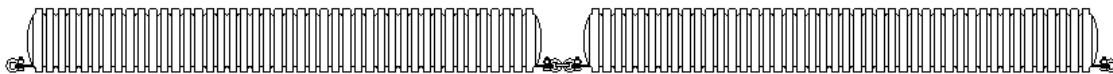
Polyethylene Corrugated Tubular Pontoons Foam Filled 12"Ø, 15"Ø, 18"Ø, 24"Ø Lengths to 20'
